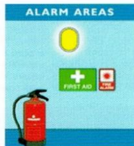
Fire alarms, first aid points and fire-fighting equipment, install within 2 metres horizontal distance.
