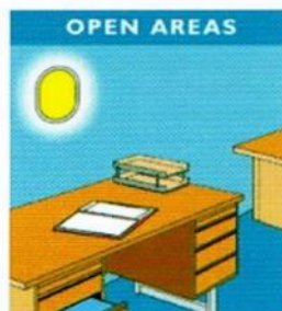
Open rooms either with a particular hazard, an escape route passing through or larger than 60m 2 .
