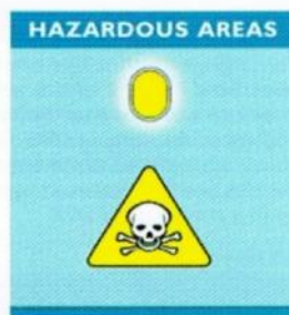
Areas of high risk should be illuminated to 10% of normal lighting or 15 lux, whichever is greater.
